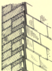
Fig. 57.—Brick Wall with Weather-tiling nailed to Fixing-blocks.
